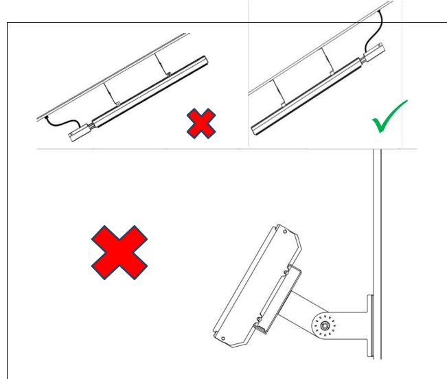
The heating surface must never be directed towards the ceiling
