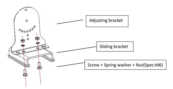
**STEP 2:** Installation of sliding bracket and heater (as arrow points).
