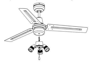
A/Get the protruding wires from base of motor. Fit fiberglass insulating sleeve over wires from the base of motor B/Get the wires with fiberglass insulating sleeve connect wires to the light kit (optional). WARNING: MAKE SURE "ACTIVE" to "ACTIVE; "NEUTRAL" to "NEUTRAL" of lampholder. Incorrect connection may cause the light to not work and may be dangerous.
