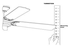
D/ Some fan movement is normal. However, interchanging an adjacent (side by side) blade pair may redistribute the weight and result in smoother operation.
