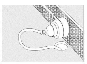
Connecting the quick set connector from remote control receiver with the connector from pre installed power code
