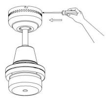
Next step. After fan is installed and hanging straight. Tighten the anti-wobble canopy bolts with pliers or wrench to Eliminate wobble during operation. NOTE: Over tightening bolts may damage canopy.
