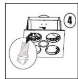
5.Now screw in the four large heat lamps into the lamp holder through the holes provided in the fascia. The globes should be screwed up firmly to ensure a good electrical contact but don't over tighten.
