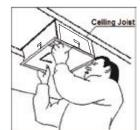
Ensure that the unit is held securely by the bar clamps
