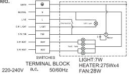
**Note**: the active and neutral wires must be connected via an all pole isolation switch with a 3mm contact clearance or a plug/socket.
