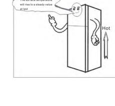
• 30 minutes later, open the freezer compartment door, feel the cold air, that means the unit works properly. After a period of time the thermostat will switch off & on automatically and set the compartments at the desired temperature.
