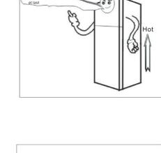
• 30 minutes later, open the freezer compartment door, feel the cold air, that means the unit works properly. After a period of time the thermostat will switch off & on automatically and set the compartments at the desired temperature.
