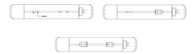
3. Fix the other two brackets onto the wall according to the distance of the bracket on the back of the unit. Drilling a round hole with 8mm diameter on the wall, place two 4 plastic plugs supplied into the hole, using the ST4 \* 35 screw to tighten the bracket onto the wall. Make sure the bracket is fixed tightly and stable.
