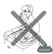
■ Do not clean the body of washer with volatile solvent such as petrol and methane. Also, do not pour these solvents into the tub for washing or drying purposes.
