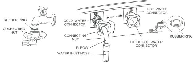
To prevent water leakage, please ensure the connecting nut is tightened securely. If water leakage, check the nut whether it is filled with rubber ring.
