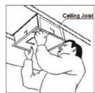
Ensure that the unit is held securely by the bar clamps
