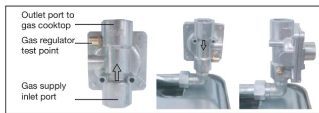
• **ULPG connection:** Using the supplied gas regulator, remove the dust seals on the inlet and outlet ports and position the outlet port of the regulator towards the gas inlet pipe of the cooktop. Using a suitable thread sealant, screw the regulator on and ensure that it is orientated with easy access to the test point. Connect the appropriate ULPG supply to the inlet port of the gas regulator.
